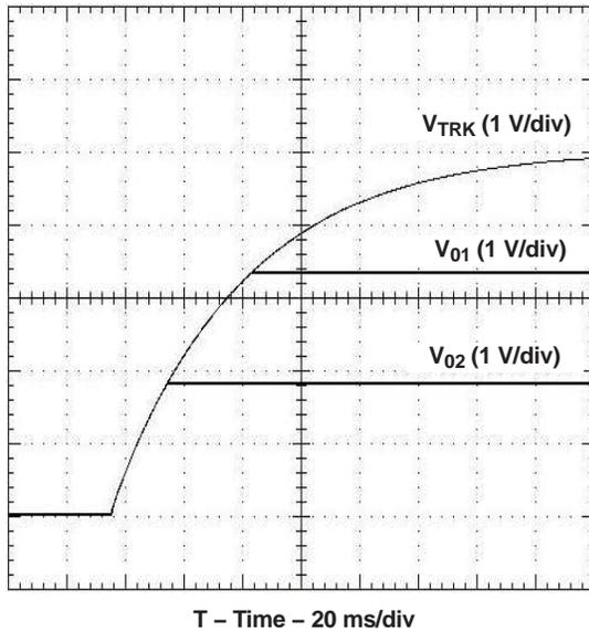
Figure 25. Simultaneous Power Up With Auto-Track Control
