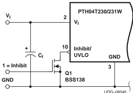
Figure 21. On/Off Inhibit Control Circuit
