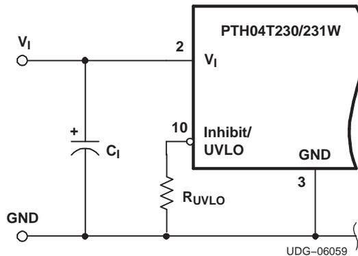
**Figure 18. Undervoltage Lockout**
