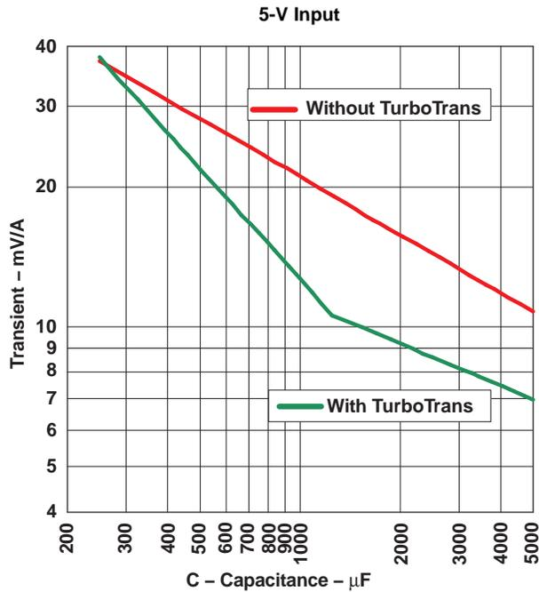
Figure 12. Capacitor Type B,  $1000 < C(\mu\text{F}) \times \text{ESR}(\text{m}\Omega) \leq 5000$
