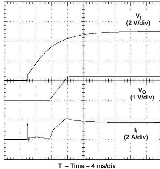
Figure 20. Power-Up Waveform
