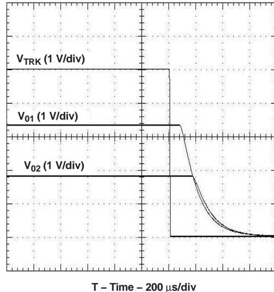
Figure 26. Simultaneous Power Down With Auto-Track Control
