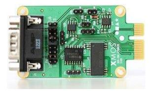
The IS-BUS sliceCARD provides flexible serial connectivity for industrial applications. It includes transceivers for CAN at 1Mbps, LIN at 20Kbps as well as a RS485 at 12Mbps, backed up by associated xSOFTip blocks. All three interfaces may be used simultaneously when connecting via the 0.1" headers. Alternatively one interface can be routed to the DB9 connector
